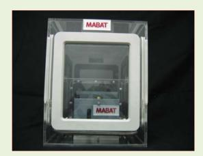
HCC-100-1 heating cooling chamber has been designed for burn-in testing. The unit can be operated and programmed from the control panel, located on the front side of electric cabinet.
