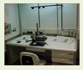
Workstation type TB-SL-2000 is use for manual eutectic soldering of components, using different soldering performs according to user standards (as Au/Ge, Ga/As etc.). The system is also allows eutectic soldering without any performs (as Silicone components soldering).
